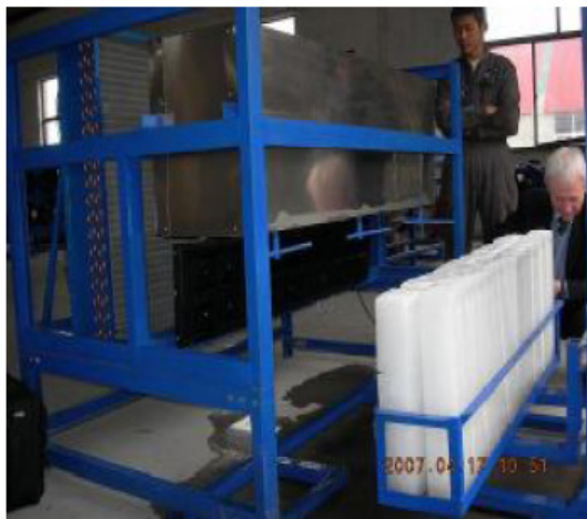
COMPACT BLOCK ICE MACHINE WITH 20 blocks every 2hours of 4.5kg each block
