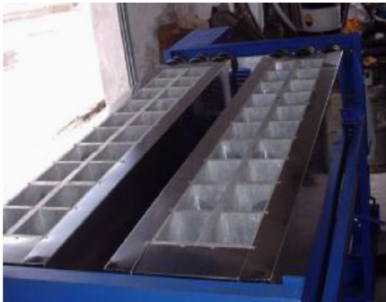
SPECIAL ALUMINUM ICE CAN WITH HIGH EFFICIENCY
