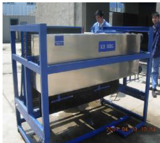
COMPACT BLOCK ICE MACHINE WITH 20 blocks every 2hours of 4.5kg each block
